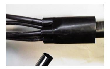
Position the cable break out.
