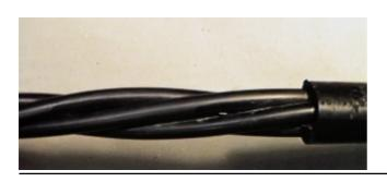
Remove the outer sheath to the necessary length for connecting to the actual equipment.
