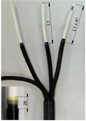
KKSI with conductive layer removed, stress controlling mastic mounted and ready for mounting of termination or connector.
