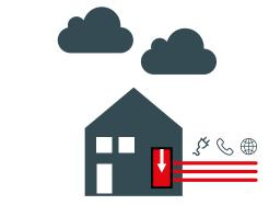
External lightning protection protects buildings in case of a direct lightning strike. It intercepts the lightning with an air-termination system, discharges and distributes it to the earth via the earth-termination system and creates a protective sheath around the building which prevents it from catching fire and protects the people within.
