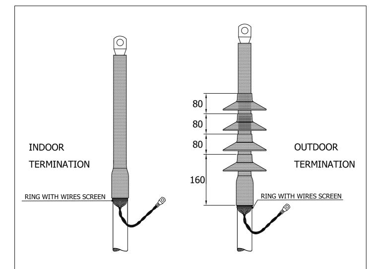
1.12 Remove the PVC tape previously applied on the screen wires and split them into two parts; wrap the wires at the bottom of shrunk tube (one round) . making a ring. Twist the screen wires, cut straight and crimp OR screw the grounding lug.
