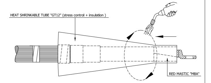
1.11 Slide the red tube "GT12" (Stress control + insulation) till the TOP edge of red mastic "MBA" applied over the cable lug and start heatshrinking from the top downwards.
