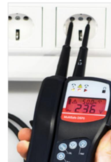
One-hand operation for testing sockets
