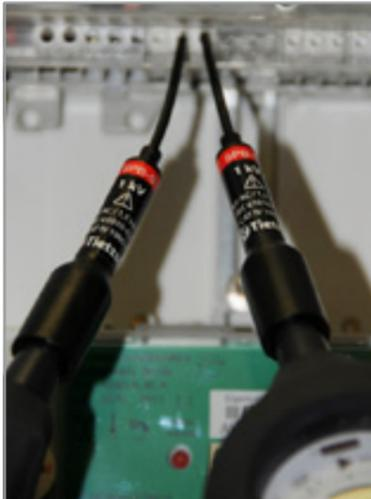
With screwed pin prods tight terminal strips or contacts at test holes can be contacted.
