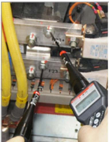
With screwed pin prods tight terminal strips or contacts at test holes can be contacted. In addition, the bare electrode length is shortened to <4 mm in order to minimize the risk of short circuits in narrow switchgear.
