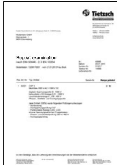
Test certificate with list of tests carried out, details of the customer and the Serial number of the test object.
