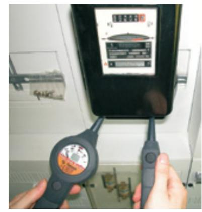
Integrated 350W-load for fast start-up tests at electricity meters
