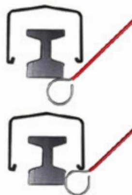
**Check on side busbars with extension and magnet**
